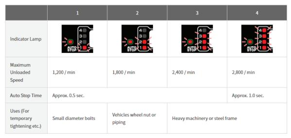
The correct tightening torque depends on the material, size and class of the bolt. Make a test fastening to adjust the mode setting to suit the bolt.
